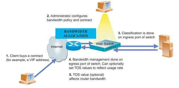
Figure 17-1 Bandwidth Management: How It Works
